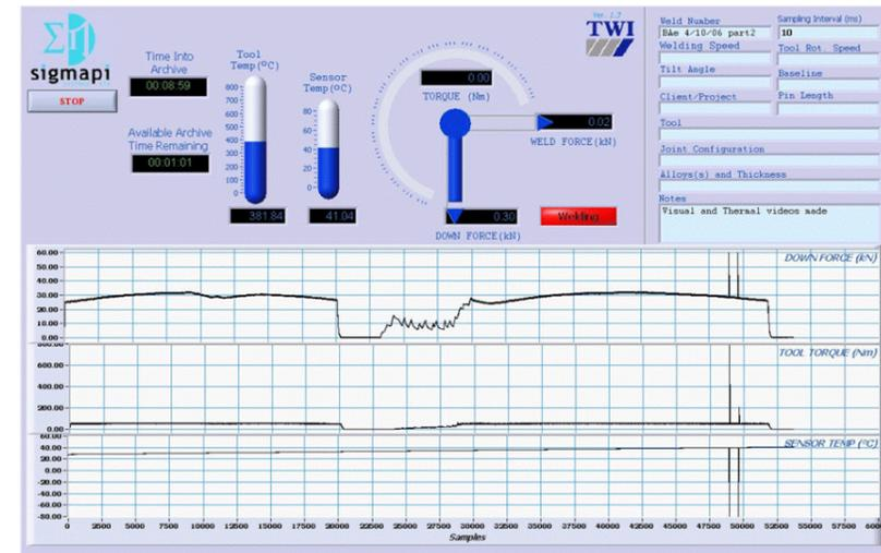
Information gathered by the LowStir sensor unit is displayed to the operator in a clear and straightforward manner using a laptop PC.
