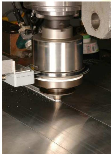
Fitting the LowStir sensor head to a milling machine is normally done with a standard ISO taper which we can supply ready connected to the head if you specify the size required (for example, ISO 50).
